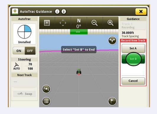
Once a line has been established, the AutoTrac button can be pressed to enable AutoTrac
